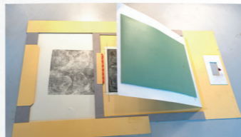
Fig. 75. A removable overlay. The rectangular hole at the top of the partially removed overlay, was located over a rectangle of thick card on the tympan to secure it.
