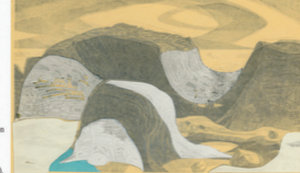
Fig. 97. An additional overlay on the set-off impression under the corner of the make-ready (reduced to 60%).
